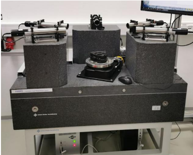
HAMS - Hurricane Angle Measurement System for ISO horizontal angle accuracy test
